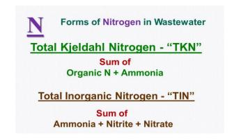
It is produced largely by deamination of organic nitrogen containing compounds and by hydrolysis of urea. At some water treatment plants, ammonia is added to react with chlorine to form combined chlorine residual.
